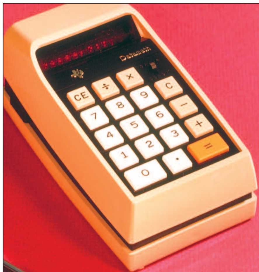
The Datamath single-chip handheld calculator, which TI introduced in 1972, was a big hit in the marketplace
